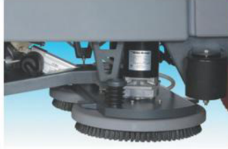
Brush release by foot. No tools required.
