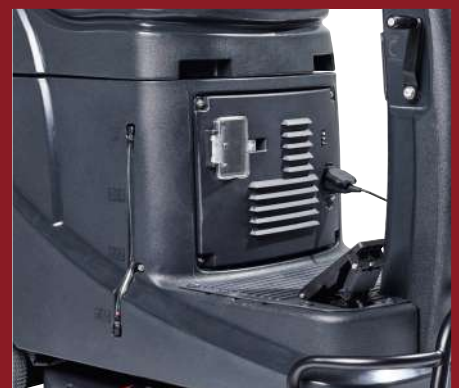
An integrated on-board charger enables easy plug-in and battery charge at any outlet
